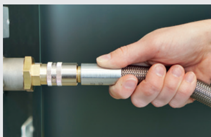
To disconnect, pull back the sleeve from the coupling (comes with automatic locking mechanism in shut-off couplings).
