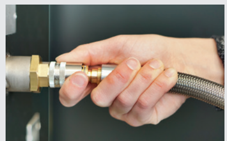
To disconnect, pull back the sleeve from the coupling (comes with automatic locking mechanism in shut-off couplings).
