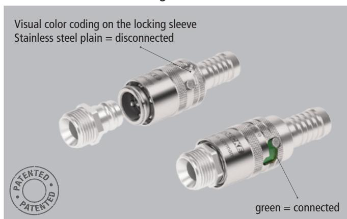
The coupling features an automatic safety locking mechanism with visual colour coding and indicates a correct and secure connection clearly and unequivocally. The disconnecting process can be blindly executed due to the forced guidance of the locking sleeve – it requires an axial movement of turning the locking sleeve, basically a manual unlocking motion.
